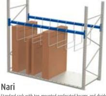
Standard rack with top-mounted perforated beams and dividers that provides access from both sides of the rack. Complete solution with bottom beams and steel shelf panel. Front-mounted rollers ease the process of loading and unloading. Section width 2700 mm. Dividers are 800 mm high and 1100 mm deep.
