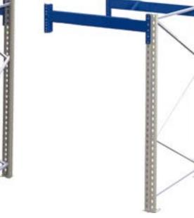
Each section can be filled with products according to your needs. A standard base section consists of 2 uprights and 2 top beams. The top beams hold the structure together but can also be used for buffer storage. An add-on section consists of 1 upright and 2 top beams. Expander bolts for concrete floors are included.
