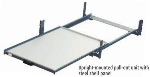
FIFO flow shelves and more accessories for upright-mounted units, see page 90–95 For goods loaded manually or with overhead crane. A steel shelf panel with 20mm high edges holds plastic bins, cardboard boxes and other items in place. Loading surface: width  $805\,\mathrm{mm}\,\mathrm{x}$  depth  $1205\,\mathrm{mm}$ .
